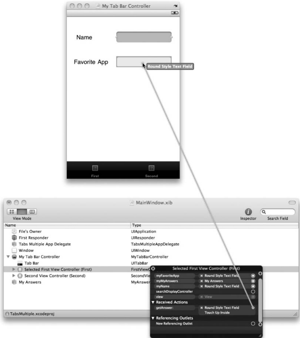
Figure 12-11 Connecting getAnswer IBAction to the text view's Did End on Exit event
