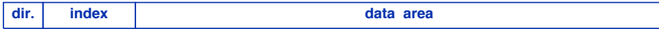
Figure 19.1 Illustration of a disk partitioned into three areas for the Xinu file system.
