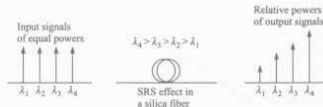
FIGURE 12-26 SRS transfers optical power from shorter wavelengths to longer wavelengths.
