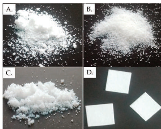
Figure 1. Pictures of carrier's beads and membranes used in BPA transformation; (A) C2C carrier, (B) C6C carrier, (C) C18C carrier, (D) CEL100 membrane.
