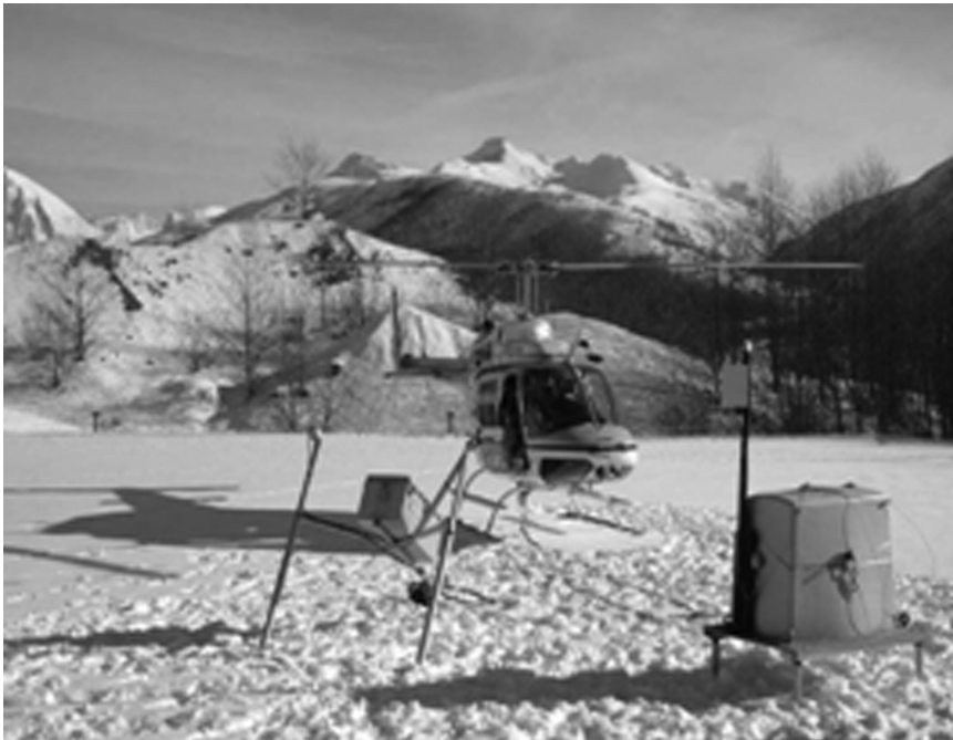
Figure 2.1 Deployment of Sensing Device by Helicopter [54].
