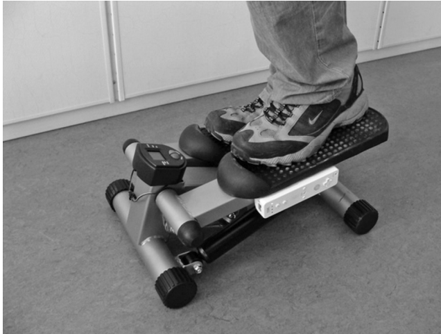
Figure 9.15 Wii Remote attached to consumer fitness device.
