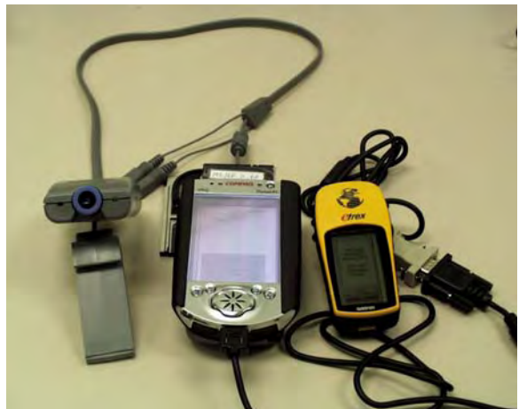
Fig. 7.2 "Smart Messages" prototype node with camera and GPS attached. (From [Iftode et al., 2004].)
