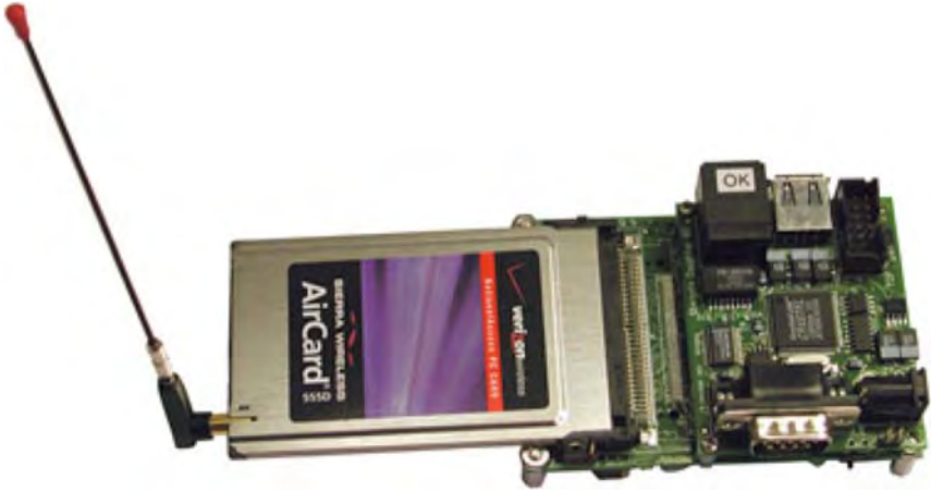
Fig. 4.9 Stargate server with a mote acting as base station. (From [Crossbow, 2006]. ©Crossbow Technology, Inc.)
