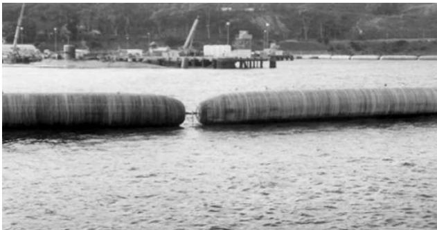
Fig. 21.1 The inflatable boom operating from a tugboat at San Diego port (photograph taken by the author)
