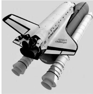
Fig. 24.1 General view of the orbiter fastened to the booster rockets
