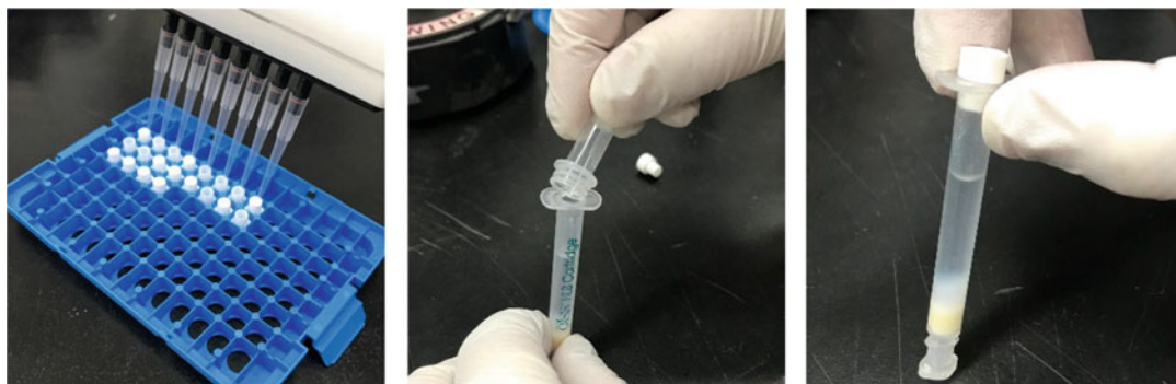
Fig. 3 Three images of iNrich method in practice. Image (left) shows NMR tube caps in 1 mL tip holder. Image (middle) describes how to pour NHS beads into an SPE cartridge. Image (right) shows a complete set of iNrich reactor plugged at both ends with a Luer plug (bottom) and an NMR tube cap (top)
