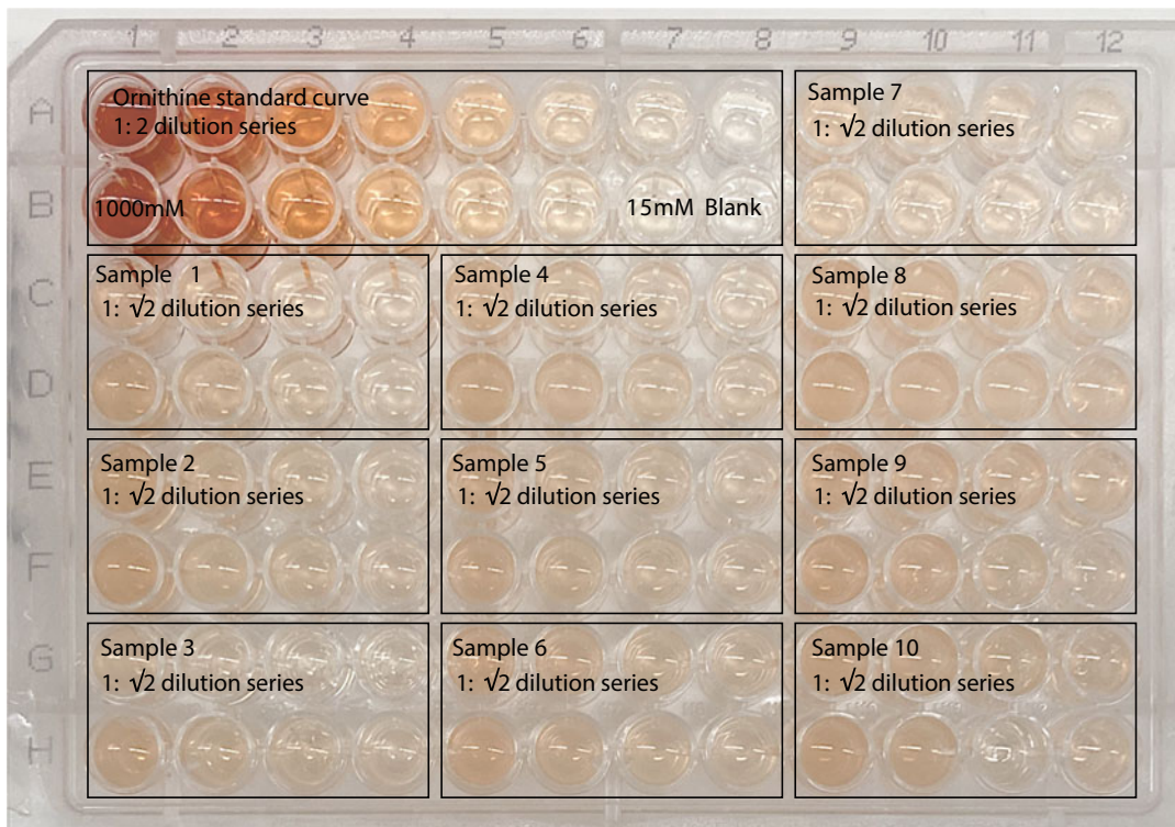
Fig. 4 Microplate layout. Plate layout for colorimetric assay, including ten patient serum dilution series and one ornithine-HCl standard curve. Standard and patient serum placement labeled on microplate
