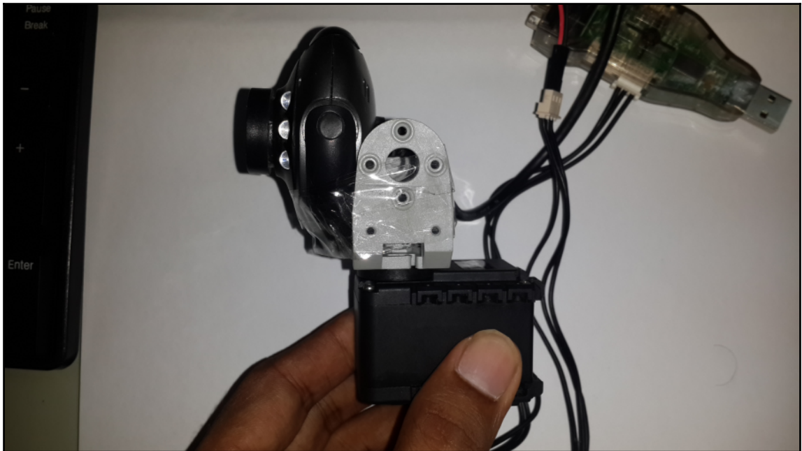
Figure 21: Fixing camera and bracket to the AX-12A
