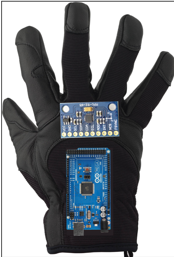
Figure 4: Hand glove with Arduino and MPU-9250
