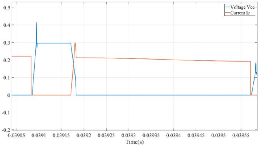
Figure 9.28 The simulation results of switching transient of switch S_a^+ (in per unit, I_{base} = 3000 A, V_{base} = 3000 V).
