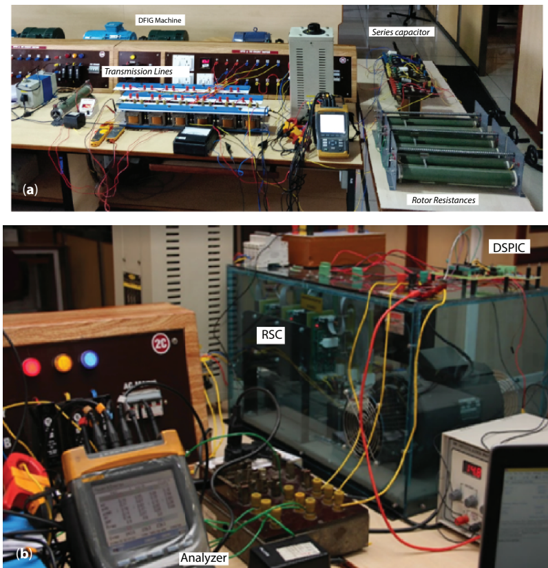
Figure 7.12 A laboratory setup of a DFIG system with a series capacitor (a) rotor circuit with Resistances; (b) RSC.
