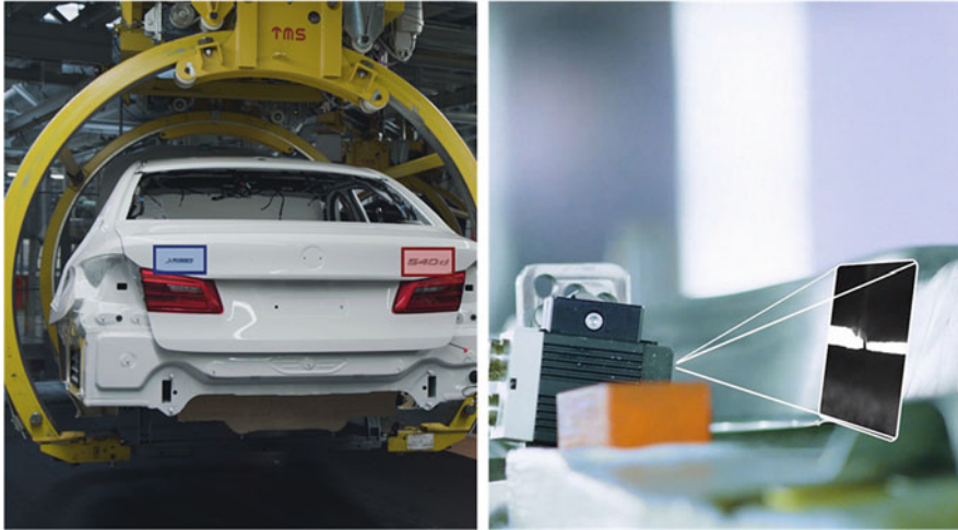
Fig. 2 AI in the BMW production system—checking the type plates (left) (BMW Group, 2019b) and tear detection in the press shop (BMW Group, 2019a)
