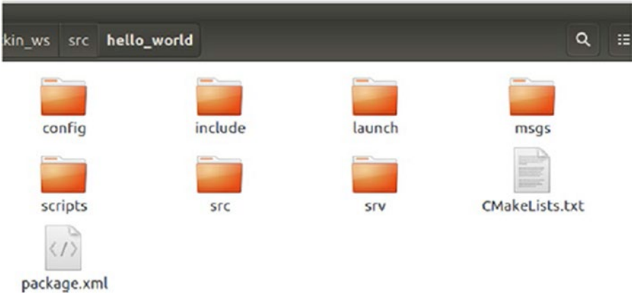
Figure 4-13. A typical ROS package structure
