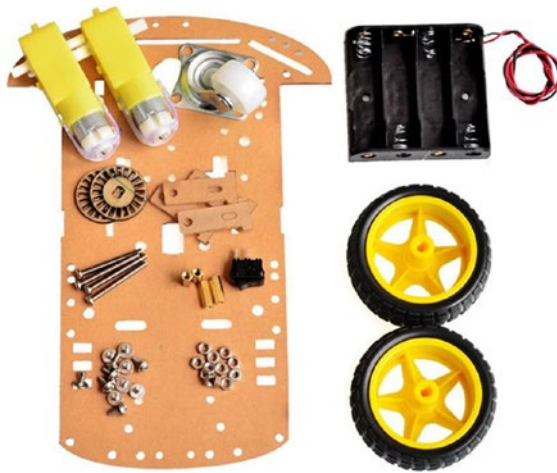
Figure 6-7. Components of 2WD robotic kit
