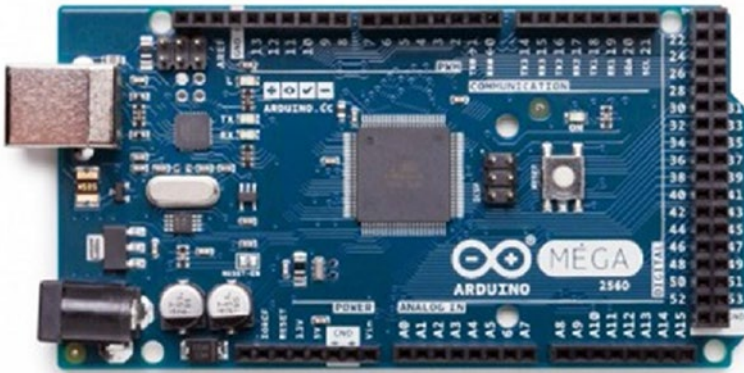
Figure 5-33. Arduino Mega 2560 board
