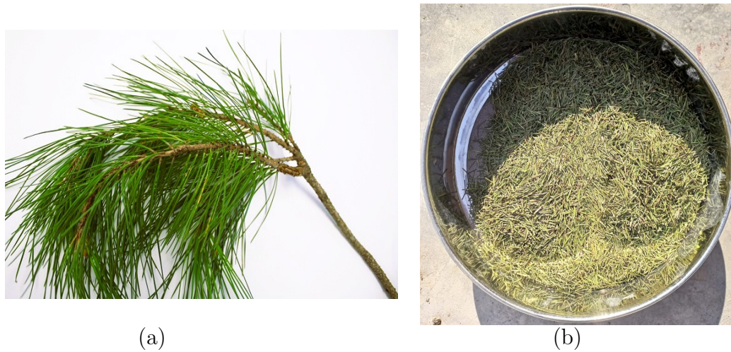
FIGURE 3.1: (a) Pine Needles in natural form (b) ALkali-treated Pine needles
