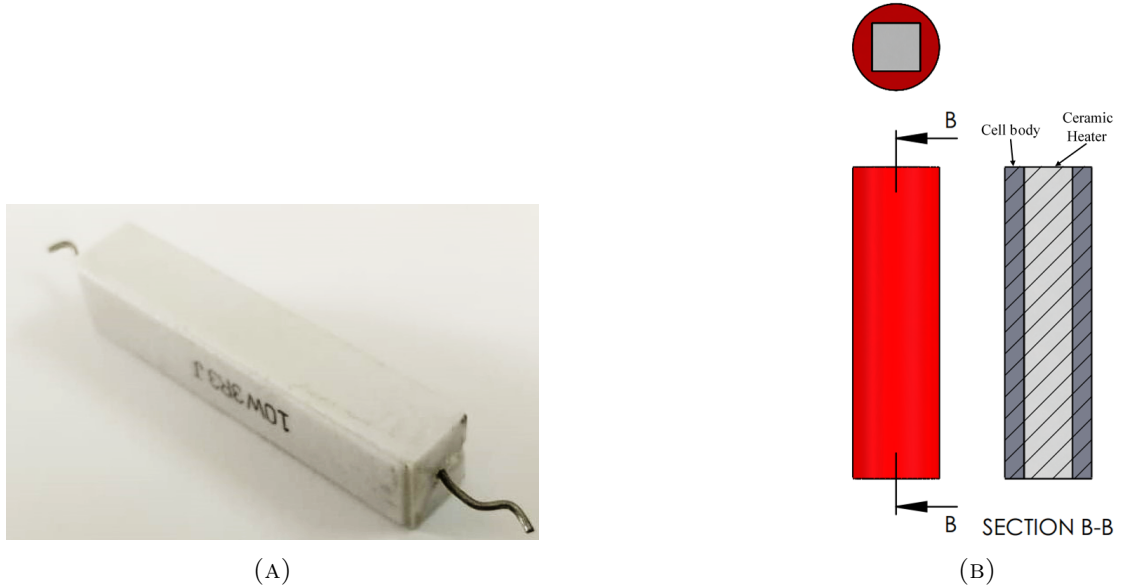
FIGURE 3.5: (A) Ceramic heater used for volumetric heat generation; (B) CAD illustration of the assembly of a ceramic heater fixed in an unfinned cell.
