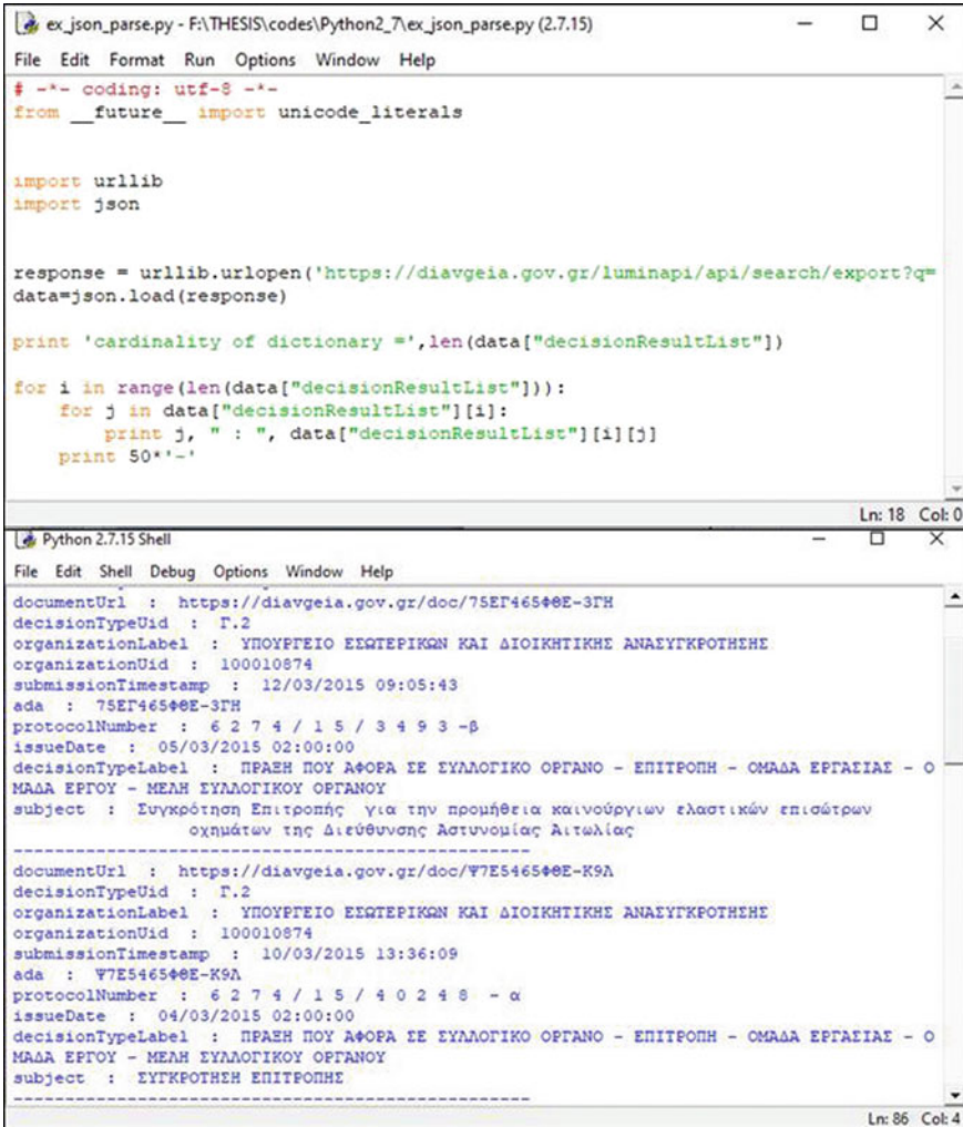
Fig. 6.20 The proposed Python code for parsing JSON data from the URL of diavgeia.gov.gr and the relevant results
