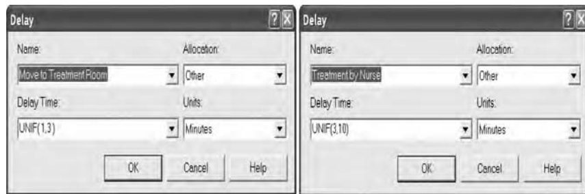
Figure 5.28 Dialog boxes of the Delay modules Move to Treatment Room (left) and Treatment by Nurse (right).
