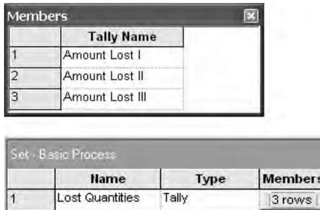
Figure 12.37 Dialog spreadsheet of the Set module (bottom) and the Members dialog spreadsheet for Tally set Amount Lost (top).
