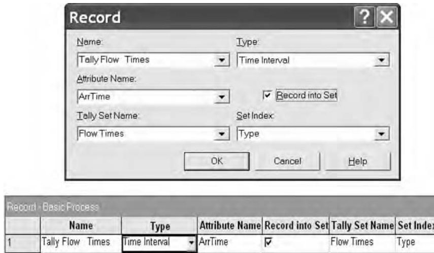
Figure 8.13 Dialog box (top) and spreadsheet view (bottom) for the Record module tallying flow times.
