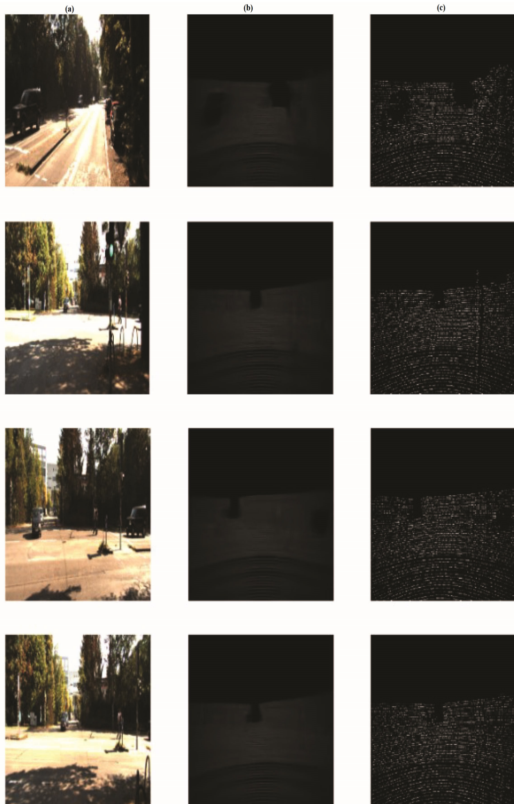
FIGURE 5.3: Resnet34 Results (30 epochs) in Dynamic Unet Configuration (without sigmoid layer) From Left to Right: (a) Original RGB image, (b) The Prediction on Validation/Test Set Images (c) Raw LiDAR Scan Data (used for training as GT).
