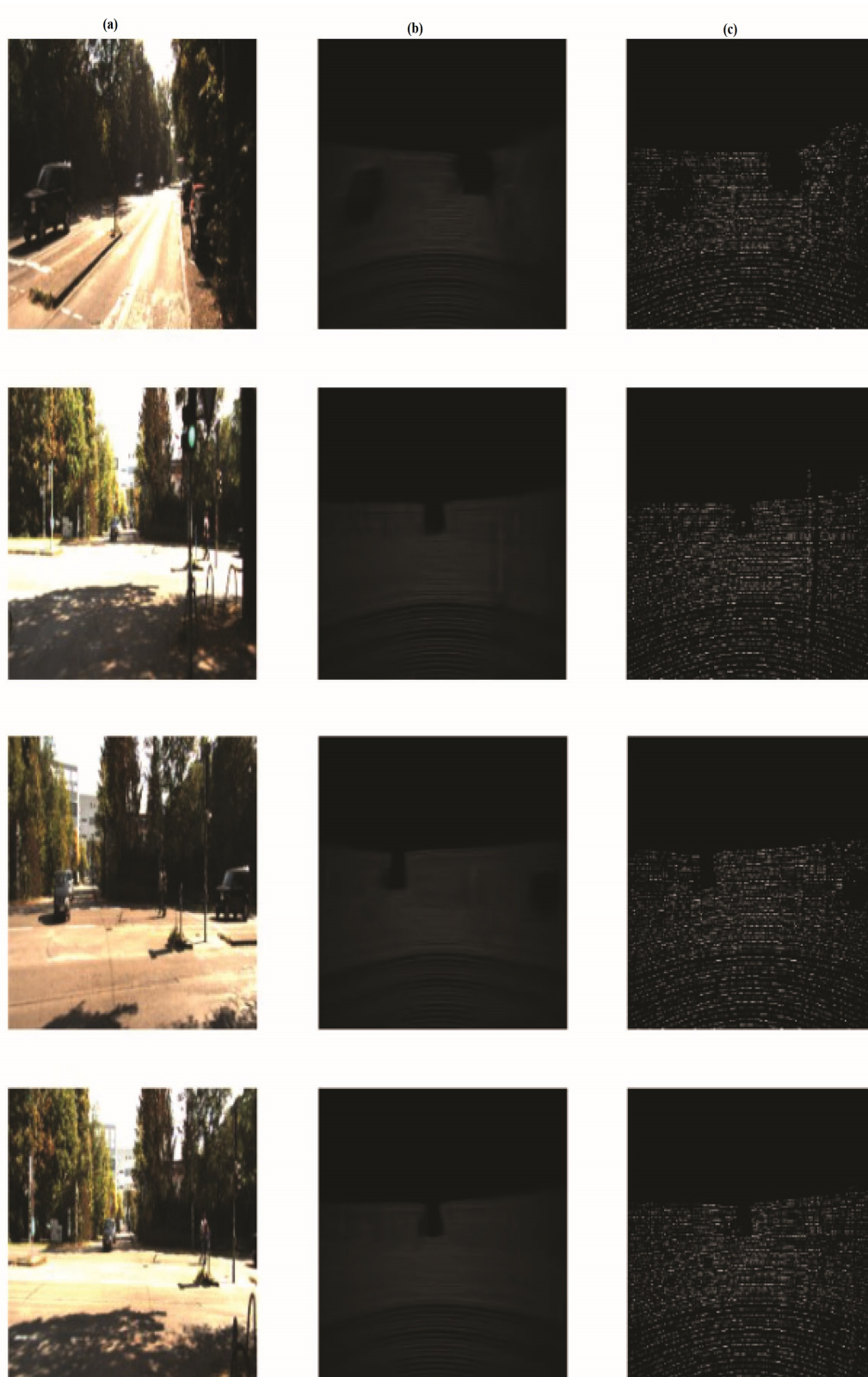
FIGURE 5.4: Resnet34 Results (40 epochs) in Dynamic Unet Configuration (without sigmoid layer) From Left to Right: (a) Original RGB image, (b) The Prediction on Validation/Test Set Images (c) Raw LiDAR Scan Data (used for training as GT).
