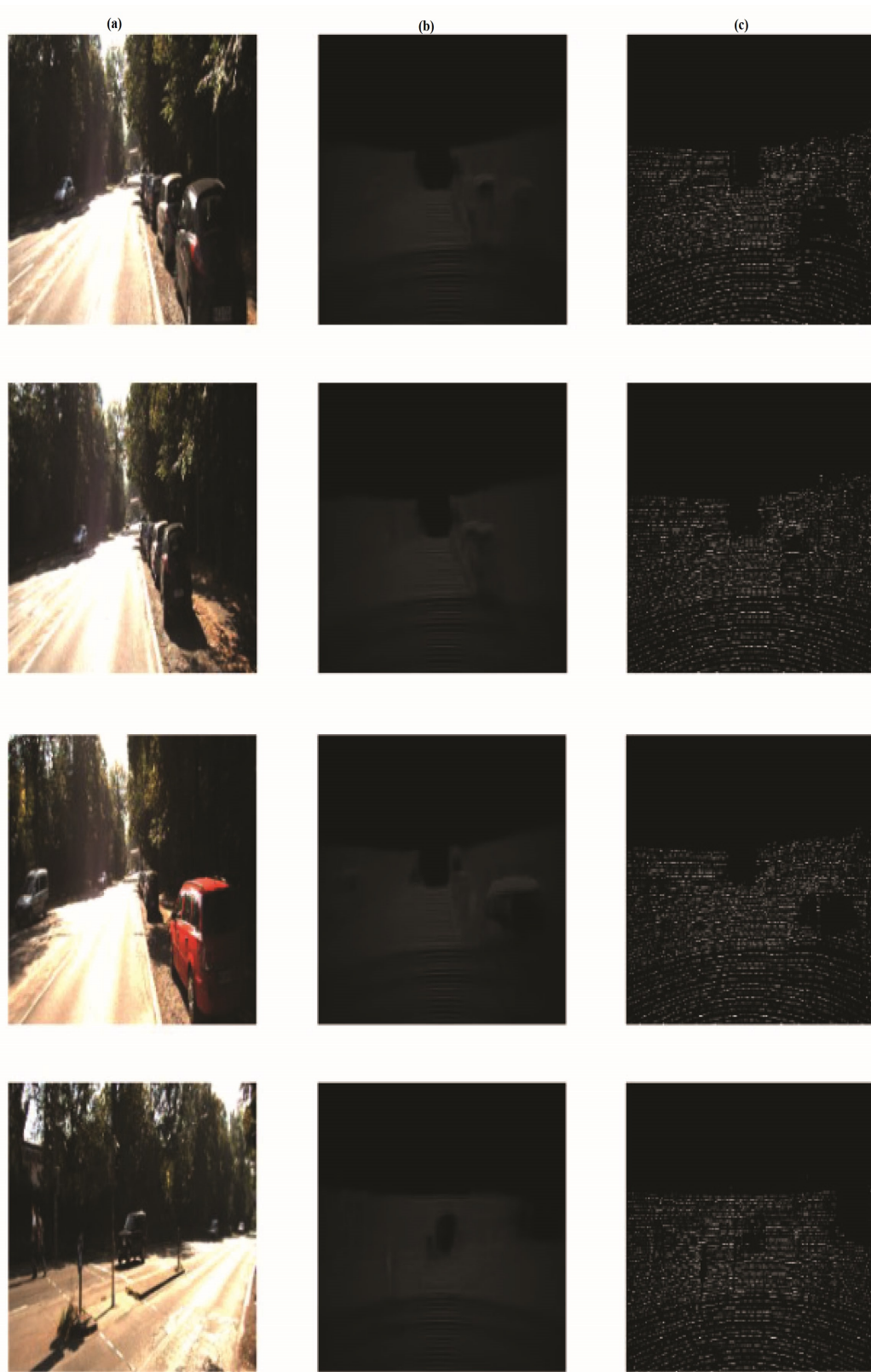
FIGURE 5.6: Resnet50 Results (10 epochs) in Dynamic Unet Configuration (without sigmoid layer) From Left to Right: (a) Original RGB image, (b) The Prediction on Validation/Test Set Images (c) Raw LiDAR Scan Data (used for training as GT).
