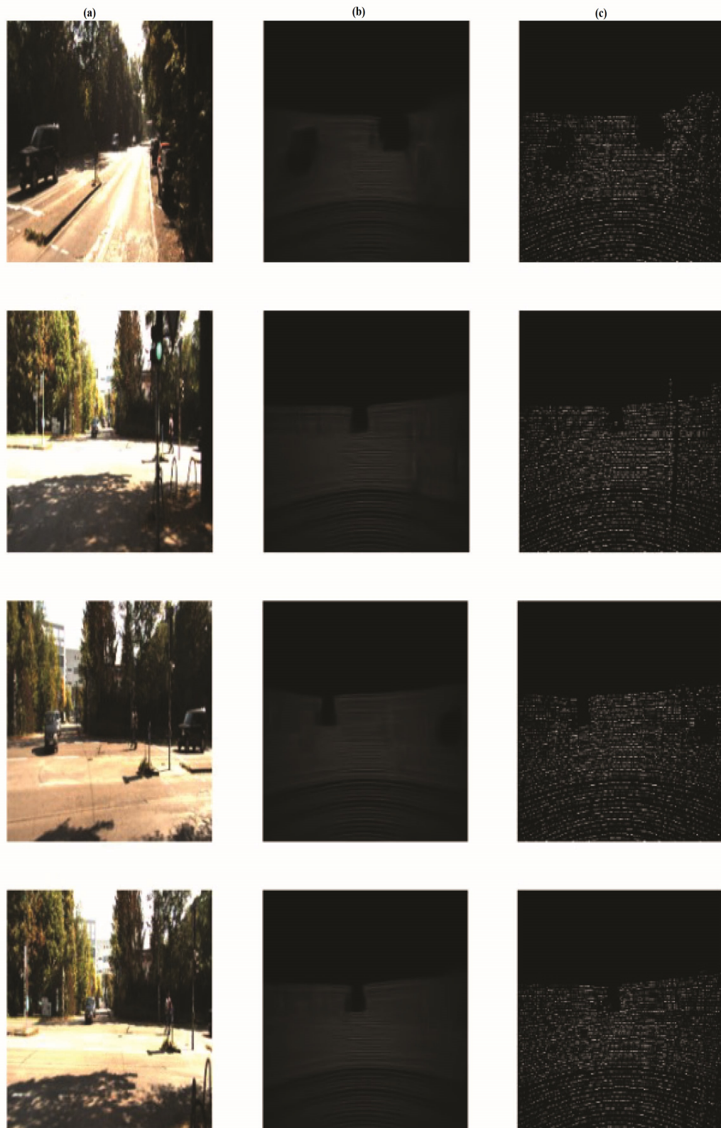
FIGURE 5.5: Resnet34 Results (50 epochs) in Dynamic Unet Configuration (without sigmoid layer) From Left to Right: (a) Original RGB image, (b) The Prediction on Validation/Test Set Images (c) Raw LiDAR Scan Data (used for training as GT).
