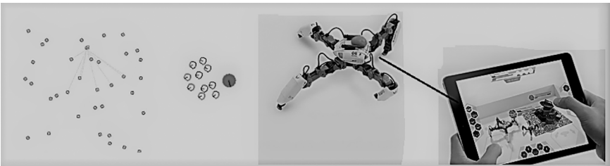
Figure 6.2 The illuminated (light-colored circle) and the occluded (dark-colored) cyborgs in swarm beacon taxis.
