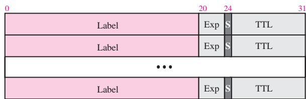
Figure 6.21 MPLS header made of stack of labels
