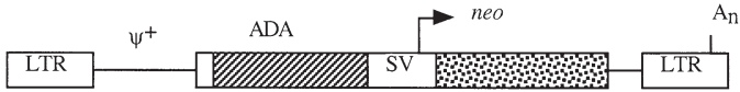
Fig. 19.3. The ADA retrovirus safe vector. LTR retroviral long terminal repeat containing the retroviral promoter and enhancer, ADA Human adenosine deaminase cDNA under the Moloney murine leukemia virus (MoMLV) promoter, SV Simian virus 40 early region promoter, neo neomycin phosphotransferase as a dominant selectable marker, \psi^+ retroviral packaging signal, A_n Polyadenylation site
