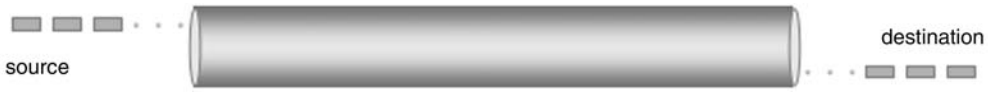
FIGURE 3.6 A flow: QoS is meaningful only for a flow between a specific source–destination pair.
