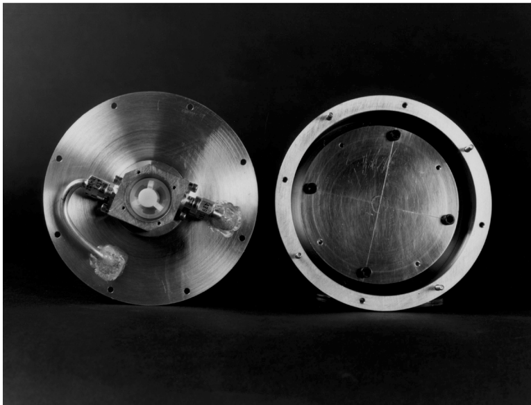
FIGURE 6.34 Illustration and photograph of the dielectric resonator probe.
