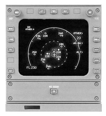
FIGURE 18.10 Joint use weather radar and traffic display.
