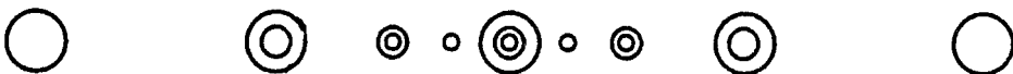
FIGURE 21.2 Three superimposed linear arrays depicted by large, midsize, and small circles. The largest array covers the low frequencies, the midsize array covers the midrange frequencies, and the smallest covers the high frequencies.
