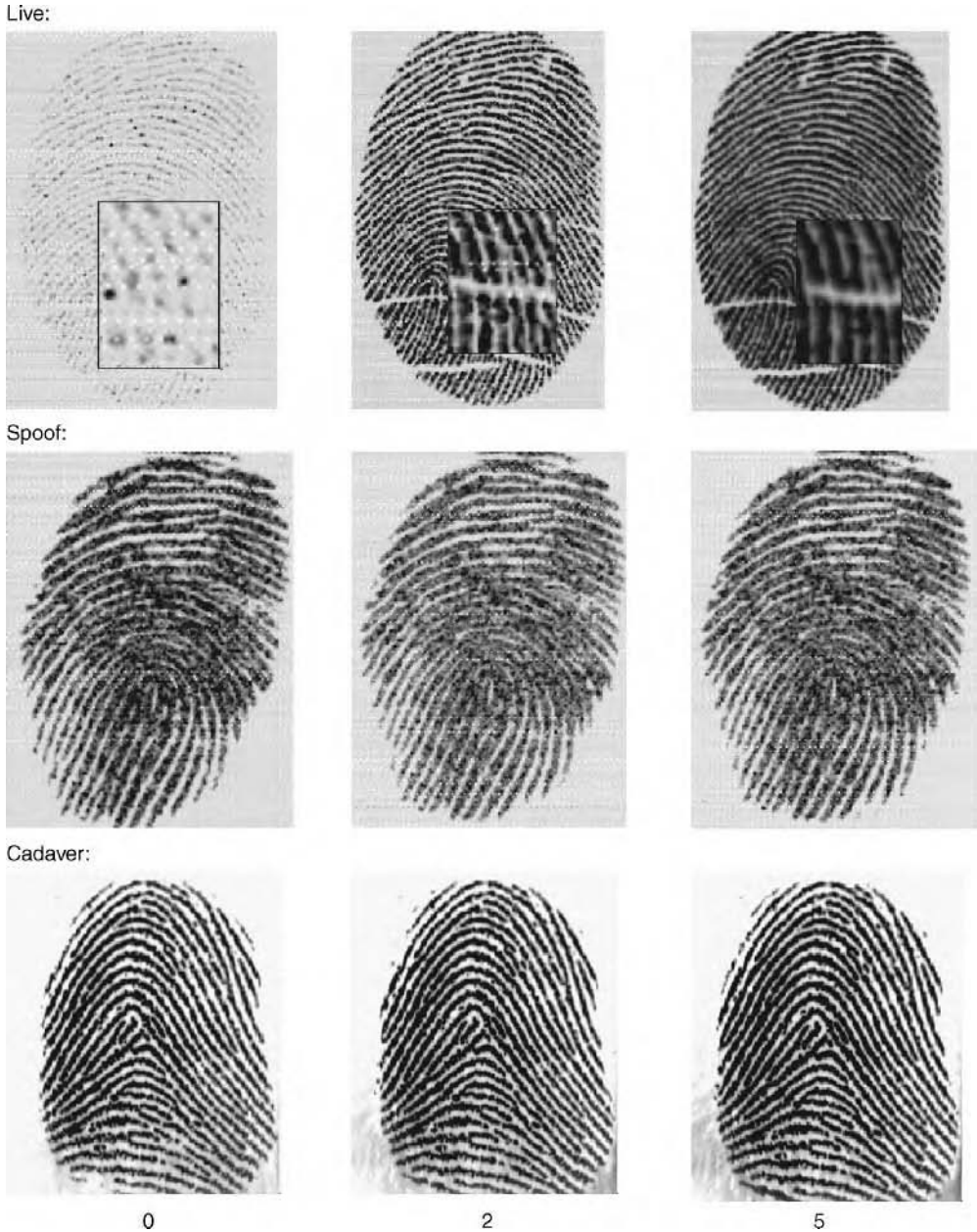
FIGURE 26.2 Example fingerprint images from live (top), spoof (middle), and cadaver (bottom) fingers captured at 0, 2, and 5 sec (left to right) after placement on scanner. Live fingerprint images demonstrate changing moisture over time due to perspiration. (Source: Parthasaradhi, S.T.V. et al., IEEE Trans. Syst., Man and Cybernetics , Part C, Vol. 35, no. 3, pp. 335–343, 2005.)
