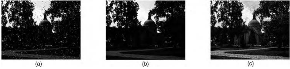
FIGURE 23.16 Image processing example: (a) original; (b) denoised; (c) histogram equalized.
