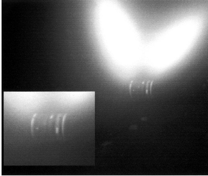
FIGURE 4.15 Typical underwater image at greater than two attenuation lengths. (Insert highlights target details.)
