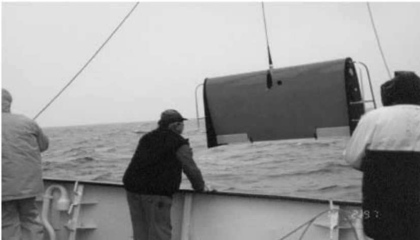
FIGURE 1.38 ScanFish MKII-IOW with SBE 911 and Fluorometer (photo by S. Krueger).
