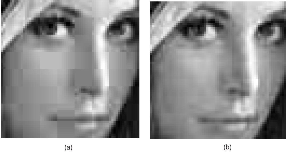
FIGURE 5.5 Zoom of image compressed using JPEG at 0.5 bits/per pixel. (a) DCT, (b) LOT. Reproduced by Special Permission of Playboy magazine. Copyright ©1972, 2000 by Playboy.
