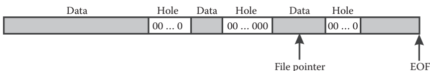
FIGURE 18.4 A UNIX file with three holes of different sizes.
