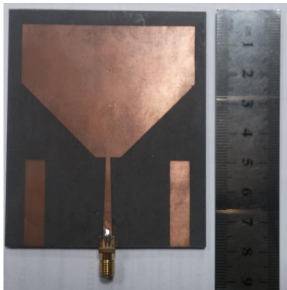
FIGURE 5.7: Prototype of the proposed hexagonal SWB planar elliptical monopole antenna.
