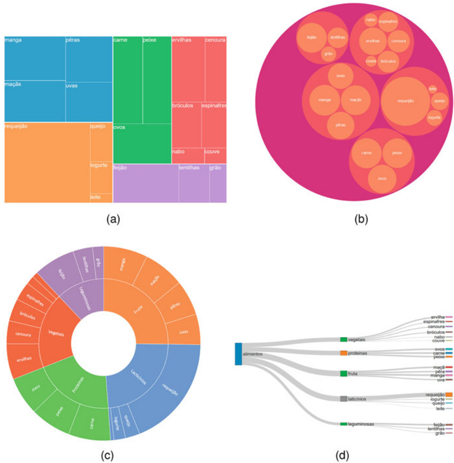
Fig. 13.1 Idioms for the hierarchy context. (a) Tree map idiom. (b) Circular packing diagram idiom. (c) Sunburst idiom. (d) Sankey diagram idiom
