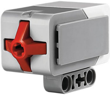
Figure 10-1. The Lego EV3 touch sensor
