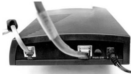
Figure 2-6 Rear view of a DSL modem showing the relative shapes and sizes of connector cables. Photo by Daly Road Graphics.
