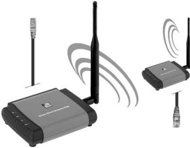
Figure 3-10 A Wi-Fi bridge can be used to extend the range or connect distant wired networks. Illustration by Daly Road Graphics.
