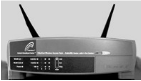
Figure 1-17 An access point, a router, a wired hub, and a firewall in one box. Photo by Daly Road Graphics.
