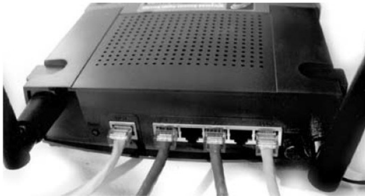
Figure 3-6 Rear view of a Wi-Fi access point with the connections to wired PCs in place. The connection to the WAN (Internet) is on the far left. A dedicated back-to-back (rolled) port for an uplink to wired hubs is on the right. Photo by Daly Road Graphics.
