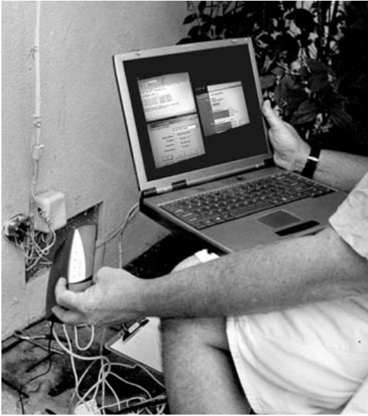
Figure 6-6 The customer disconnects his house phones entirely and sets up his DSL modem directly to the incoming phone line. Photo by Daly Road Graphics.
