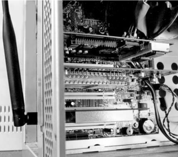
Figure 3-7 A workstation's Wi-Fi antenna is parallel to a metallic surface. Photo by Daly Road Graphics.
