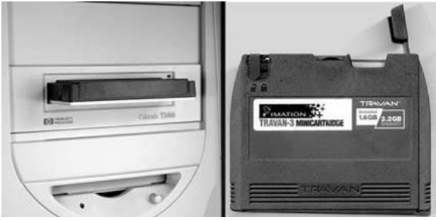
Figure 5-2 A built-in backup tape drive and one of the cartridges that it uses. Photo by Daly Road Graphics.
