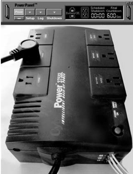
Figure 5-5 Above: The UPS can be controlled from the PC screen and vice versa. Below: A small UPS with additional sockets for phone line spike suppression. Photo by Daly Road Graphics.
