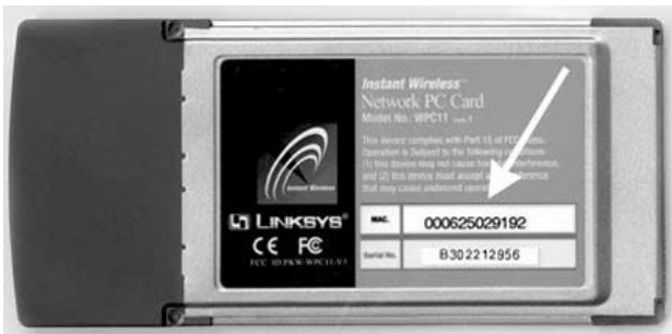
Figure 4-5 A sample MAC, as shown on the underside of a PCMCIA Wi-Fi card. Photo by Daly Road Graphics.
