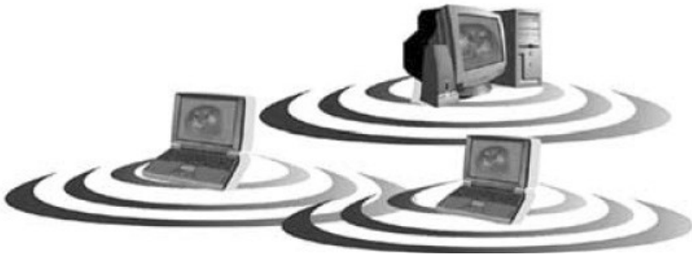
Figure 3-4 In ad hoc mode, every station connects to every other. Courtesy of Linksys.
