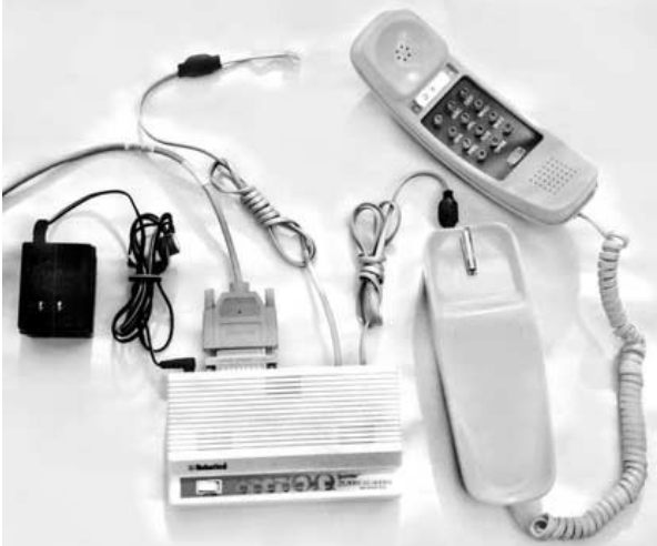
Figure 1-1 A standard modem, the old way of connecting to the Internet. Photo by Daly Road Graphics.
