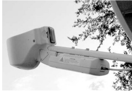
Figure 2-2 A close-up of a satellite Internet dish's feeder horn. Photo by Advanced Network Systems.
