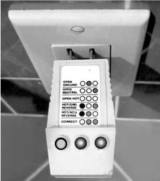
Figure 5-3 The indicator lights tell you at a glance if your power outlet is miswired. Photo by Daly Road Graphics.
