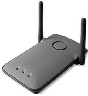
Figure 1-16 A typical, simple Wi-Fi access point. Photo by Belkin.
