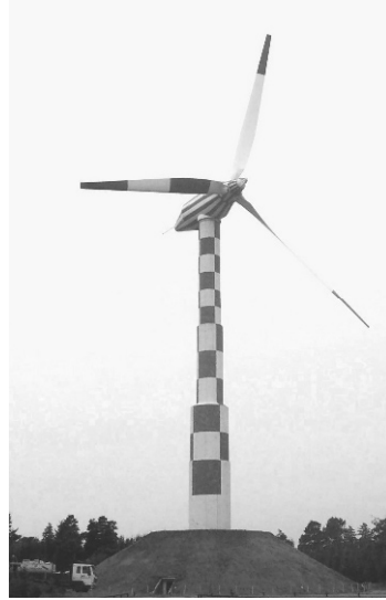
b) TVIND wind turbine (2,000 kW, D = 54 m, DK 1977)
