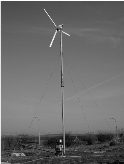
Fig. 3-57 Left: guyed pole (Aerosmart 5); right: mobile hybrid system (Terracon Energy Container)
