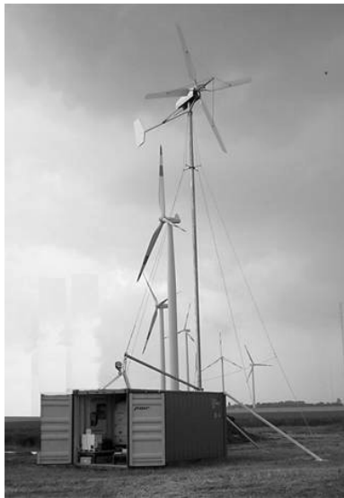
Fig. 3-57 Left: guyed pole (Aerosmart 5); right: mobile hybrid system (Terracon Energy Container)
