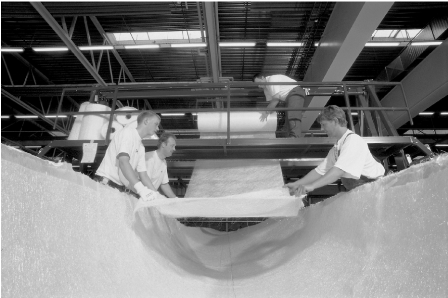
Fig. 9-14 Manufacturing of rotor blades at LM, DK; laying of the glass fiber fabrics
