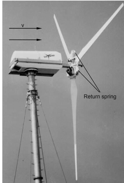
Fig. 3-18 Wind turbine SÜDWIND 1237, downwind rotor with flapping hinge
