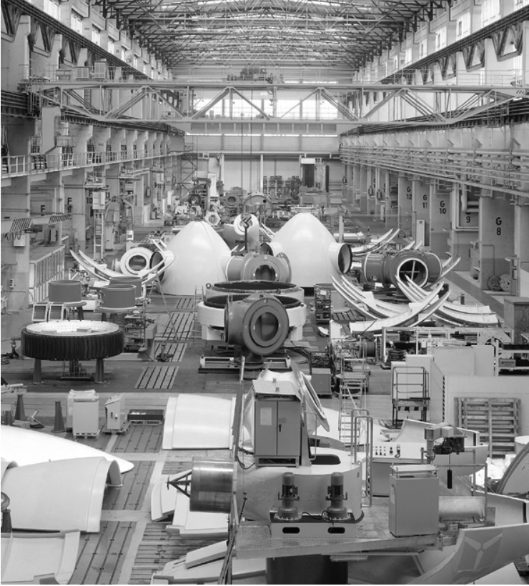
Fig. 3-61 Nacelle assembly shop at company ENERCON
