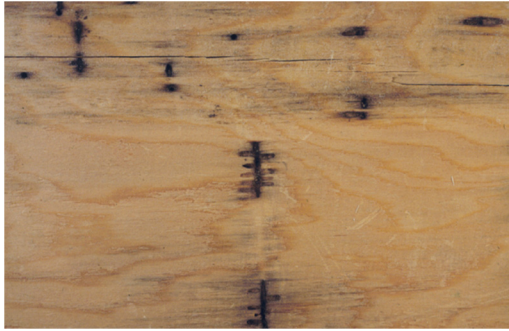
Figure 2.4 Stain and tunnels (pinhole galleries) damage in soft maple lumber caused by attack of ambrosia beetle ( Trypodendron lineatum Oliver) after the tree was cut. Most ambrosia beetles invade dying trees, slash, or green roundwood. Ambrosia beetle attack is sometimes confused with decay if the tunnels are not obvious.
