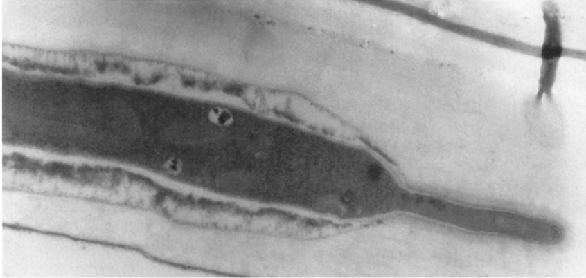
Figure 9.8 TEM of a Type 1 soft rot cavity produced by Phialophora hoffmannii in Betula pendula showing a diamond-shaped cavity with fine proboscis hyphae and halo surrounding the hyphal tip and the tip of the hyphal cavity prior to. From Hale, M.D., Eaton, R.A., 1981. Soft Rot Ultrastructure . The International Research Group on Wood Preservation Document No IRG/WP/1138. Stockholm, Sweden.
