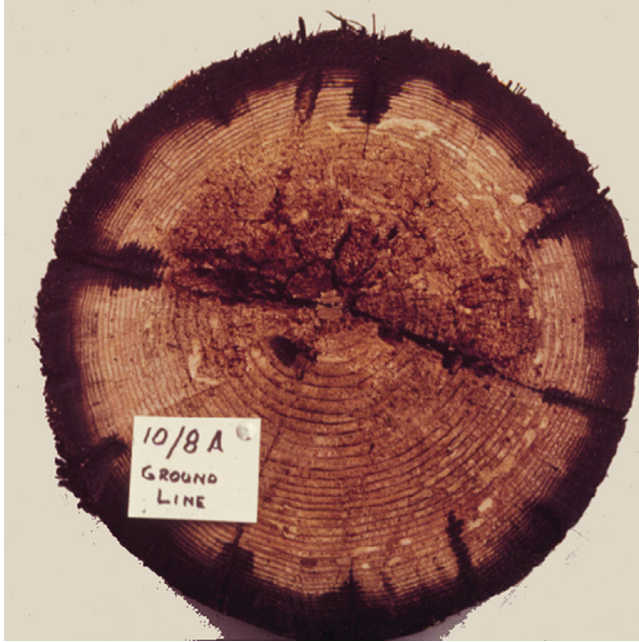
Figure 15.7 A cross section in the groundline zone of a treated Douglas-fir transmission pole indicating the association between deep checking (arrows) and the development of internal decay. Courtesy: R.W. Meyer.
