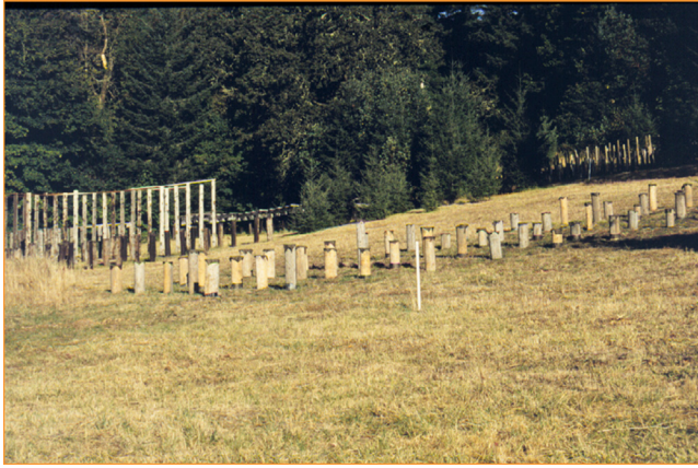
Figure 19.7 A section of a large field installation of treated pole-diameter posts evaluating various wood species and treatment methods. The test site is located near Corvallis, Oregon.
