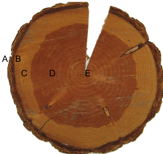
Figure 6.1 (A) Cross section (transverse) of a Douglas-fir stem ( Pseudotsuga menziesii ) stem showing the (A) bark, (B) cambial zone, (C) sapwood, (D) heartwood, and (E) pith zone.
