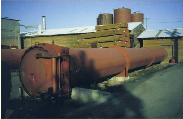
Figure 19.1 Commercial wood treatment cylinders (retorts) can range from 1.5 to 4 m in diameter by up to 42 m in length.
