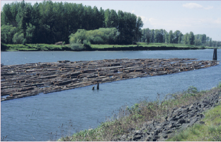
Figure 13.3 A large raft of logs in the Pacific Northwest assembled for water protection against insects and fungi.
