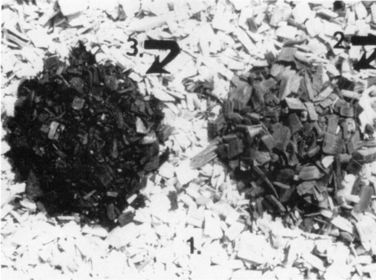
Figure 13.6 Examples of heat/acid damaged wood chips caused by improper storage on top of fresh chips. The small pile on the right was exposed to temperatures in excess of 175 °F for 3–4 weeks, the pile on the left was exposed to the same temperatures for 6–8 weeks and smelled of acetic acid. Courtesy W.S. Fuller, Weyerhaeuser Co. and permission TAPPI (1985).
