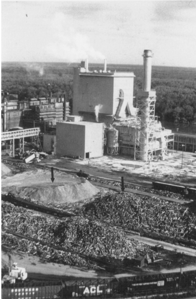
Figure 13.5 A large pulp mill showing the large piles of chips and pulpwood bolts required to maintain a constant supply. Courtesy W.S. Fuller, Weyerhaeuser Co. and permission TAPPI (1985).
