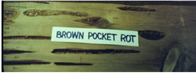
Figure 12.3 Example of the typical brown cubical pocket rot on cypress, known in the lumber trade as “pecky cypress”.
