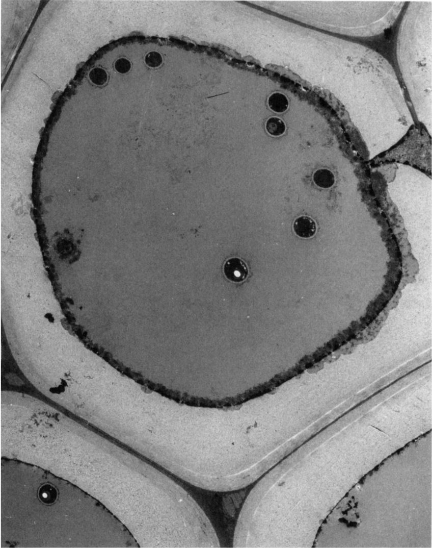
Figure 9.7 TEM of CCA treated Betula verrucosa after a one-month exposure to Phialophora mutabilis showing erosion of the S-2 cell wall layer away from fungal hyphae as well as CCA residue along the S-3 cell wall layer. From Daniel, G.F., Nilsson, T., 1989. Interactions between soft rot fungi and CCA preservatives in Betula verrucosa . J. Inst. Wood Sci. 11 (5), 162–171.
