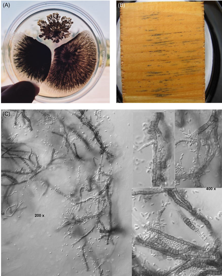
Figure 17.1 Some macroscopic and microscopic features of Aureobasidium pullulans showing (A) a colony on malt extract agar, (B) the fungus discoloring a wood sample, and (C) a composite of microscopic images showing hyaline hyphae, conidiogenous cells, and pigmented conidia. All images courtesy of FP Innovations.
