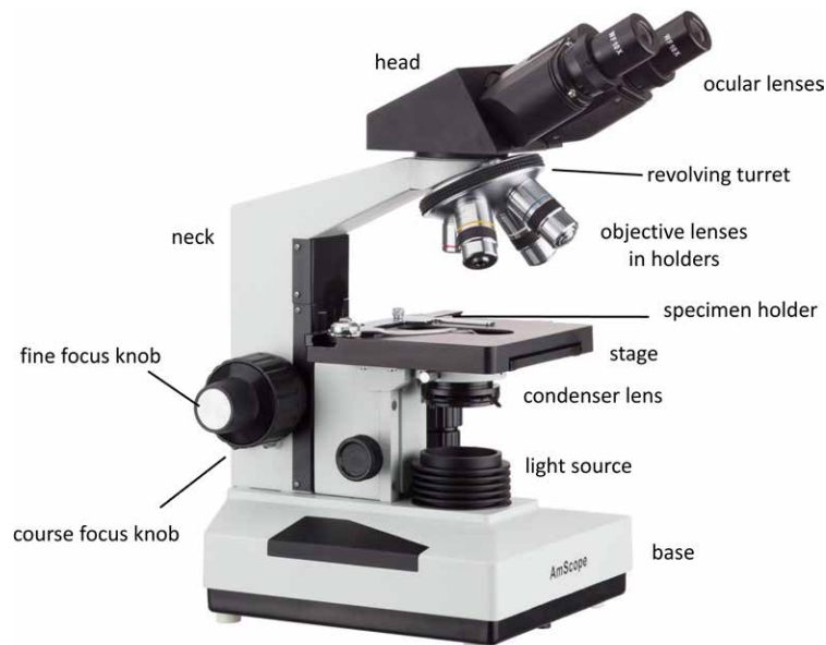
Figure 1-6 Major parts of a modern microscope. Photograph courtesy AmScope.
